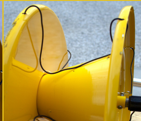
wire tie off for wire being rolled
