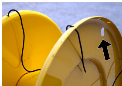
Wire tie off for wire being rolled.
